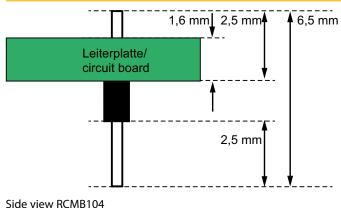
Recommended drilling diameter: ø 1,1 mm
